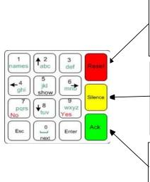
This resets the panel after an alarm condition. All initiating devices are reset, and the panel is cleared of any alarm conditions. If an initiating device is still in alarm after the system is reset, such as a smoke detector continuing to sense smoke, or a manual pull station still in an activated position, another alarm will be initiated.
